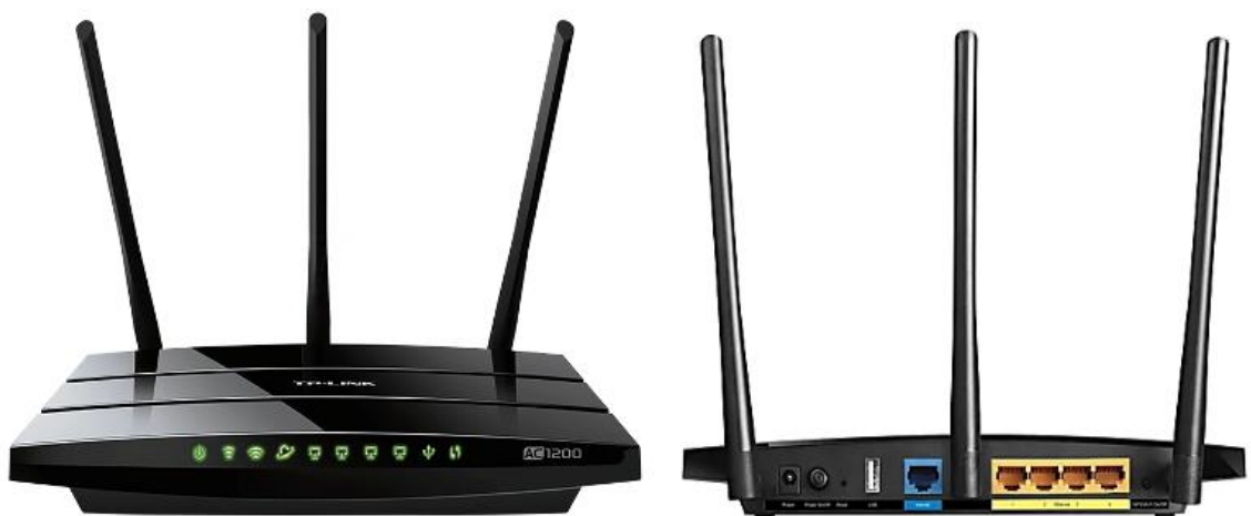
Figure 6: Front and back image of the TP-Link Archer C1200 showcasing ports and power connections [11].
