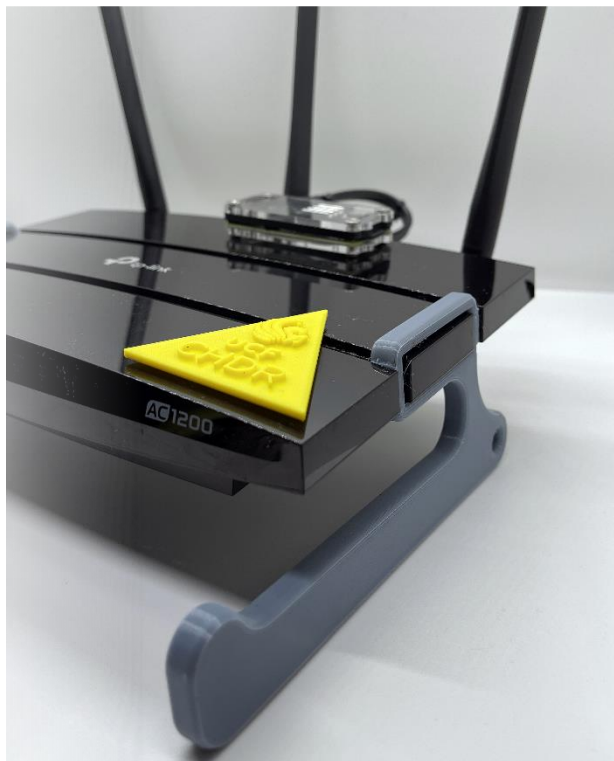
Figure 10: 3D Printed Arms attached to the side of the router.
