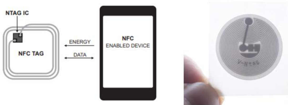
Figure 13: From left to right, Diagram of NFC Functionality from NTAG 215 Manual and Actual photo of NTAG 215 NFC Tag
