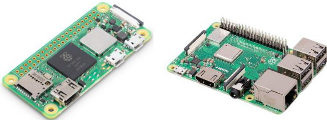
Figure 4: From left to right, Pi Zero 2 W and Pi 3 B+
