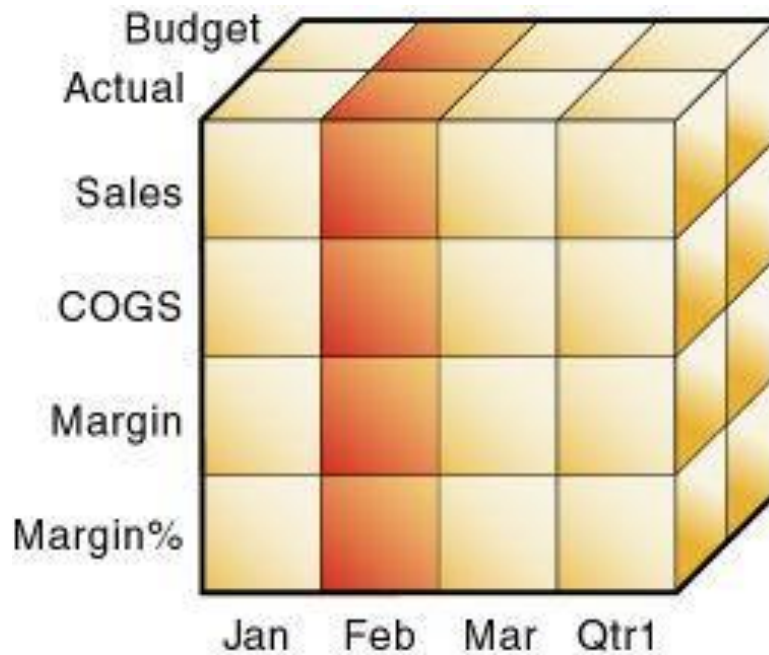
Figure 8.1.3.10.2: This is a diagram of the use of a view to show the information in this particular database pertaining to the month of February. As is demonstrated here, views can be used to show specific subsets of the database, and in this case, the user can only see the information pertaining to February and not to January.
