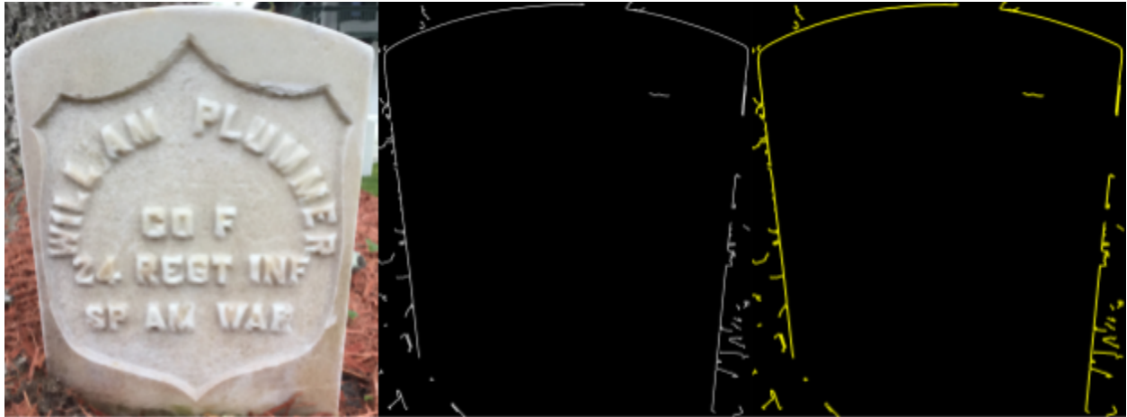
37 A picture of a headstone that has gone through three major cv2 operations: closing, canny edge detection, and contour detection, respectively.
