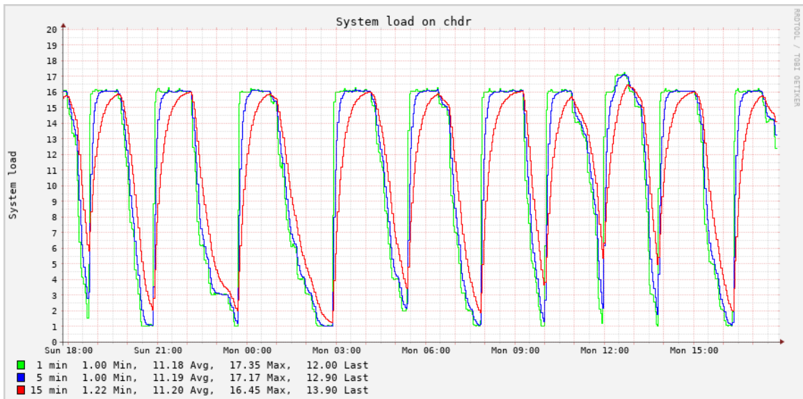
Figure 86: System load of last 24 hours of automatic quick lookup. The huge dips in system load are likely due to outliers – quotes that take a much longer time to search for than the rest. The algorithm currently waits until all the quotes in the current chunk that it is performing a multiprocessed search on are finished until moving onto the next quote, so that explains these dips.
