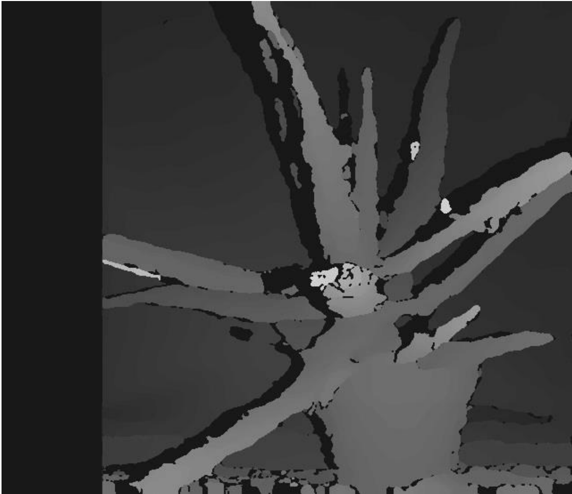
Disparity map calculated from the two images
