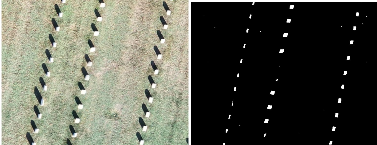
Figure #: Example of how a tool might be able to see gravestones easily and detect their areas
